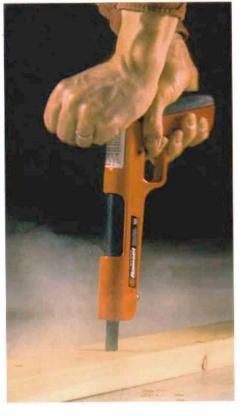
Working with steel and concrete is easier with powder-actuated tools. Modern PATs are guieter and faster, with semiautomatic and fully automatic functions that allow nearly nonstop firing.
